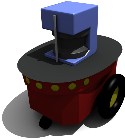
Figure 3.2: Pioneer 2 equipped with laser scanner and retroreflective beacon.
