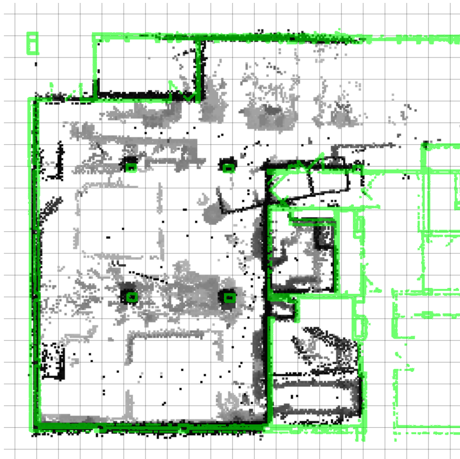
Figure 6.9: All scans for the trajectories in Figure 6.10, aligned using the iterative multi-resolution scan matching algorithm. Angular resolution of matching is carried out at 0.25^\circ . The occupancy map has a cell resolution of 0.08m and includes 20 scans from each of the four robots. Higher voxels are darker. The ground truth schematic is superimposed in green.
