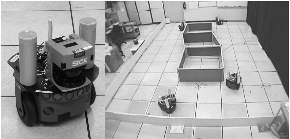
Figure 6.2: A team of Pioneer 2DXs used by Howard et al. (2003) equipped with SICK LMS200 scanning laser range finder and pair of retroreflective cylinders
