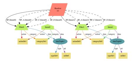
Fig. 6. A Positive Test Case for Behavior Testing
