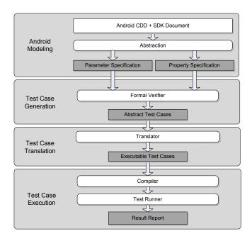
Fig. 1. Model-based Conformance Testing Framework
