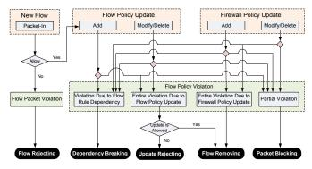
Figure 1: FLOWGUARD violation resolution mechanism.
