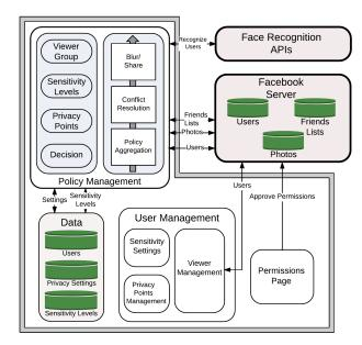
Figure 4: System Architecture of AppX.
