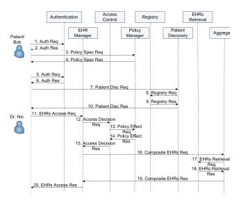
Fig. 6: System Workflow
