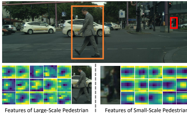
Figure 1: Visualization of ROI feature maps from a large-scale and a small-scale pedestrians. In our implementation, the ROI features of a pedestrian have 7 \times 7 \times 256 dimensions. Each feature map shown above is selected from the 256 feature channels.
