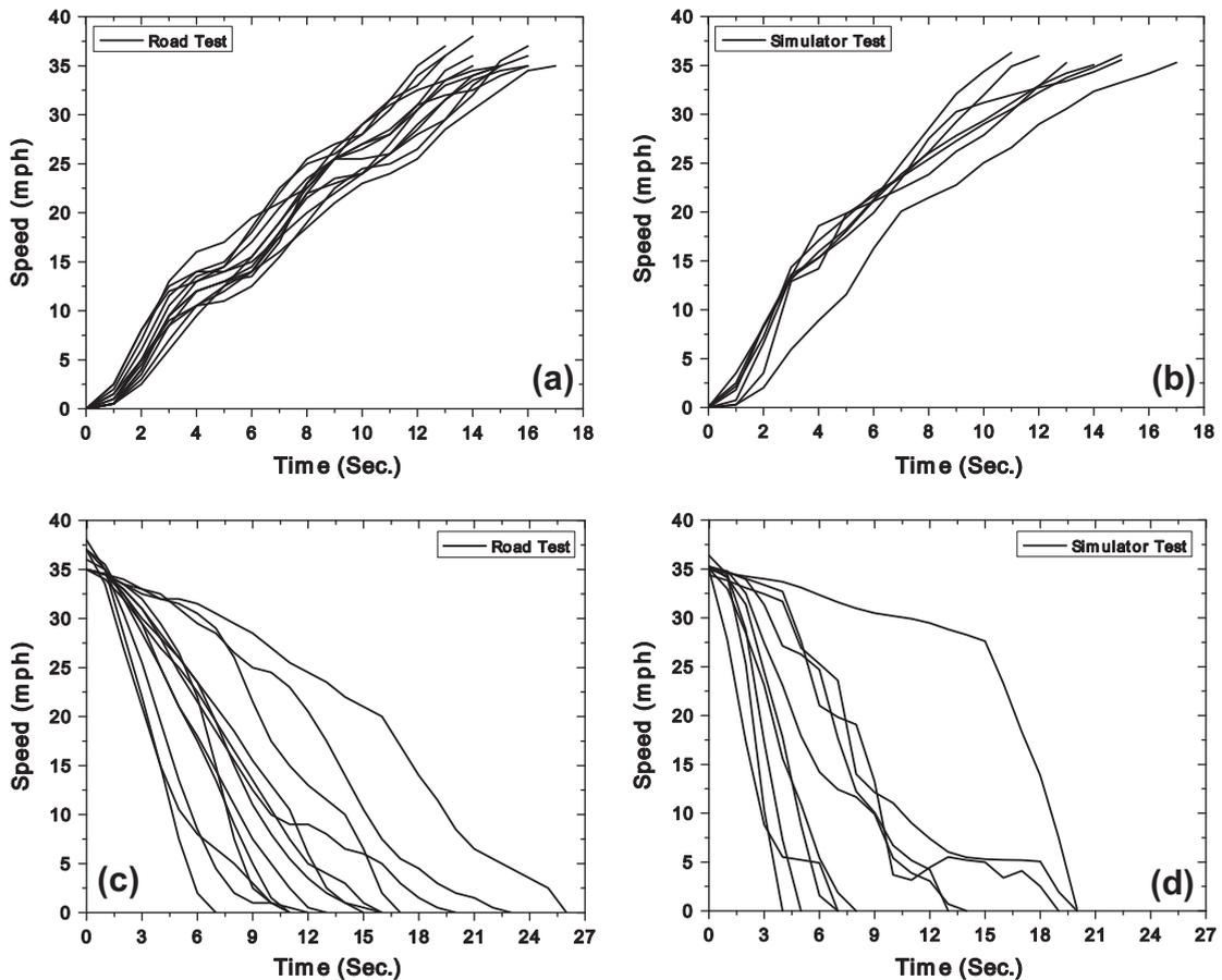
**Fig. 4.** (a–d) Acceleration and deceleration profiles for a given participant.
