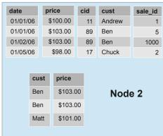
Figure 1: Relationship between tables and projections. The sales tables has 2 projections: (1) A super projection, sorted by date, segmented by  $HASH(sale\_id)$  and (2) A non-super projection containing only (cust, price) attributes, sorted by cust, segmented by HASH(cust).
