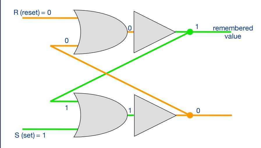
Because the output of the bottom OR gate will now stay at 1, we can lower S to zero, and the circuit will stay in a stable state, with 1 as the remembered value!
