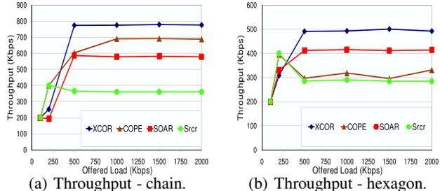
Figure 2: Throughput comparison of Srcr, SOAR, COPE, and XCOR in two different topologies.
