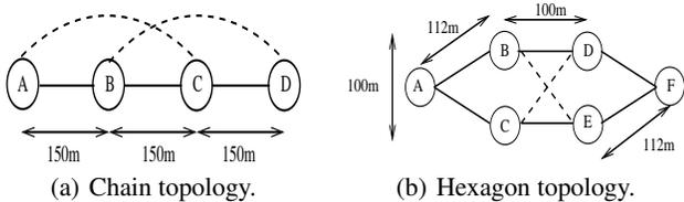
Figure 1: Two topologies used in simulation evaluation.
