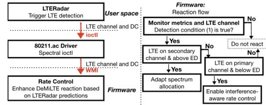
Figure 12: System architecture with LTERadar (left) and reaction flow of *DeMiLTE* (right).
