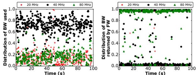
Figure 4: Chosen bandwidth by Wi-Fi AP in hardware (left) and firmware (right), when LTE is on secondary channel.
