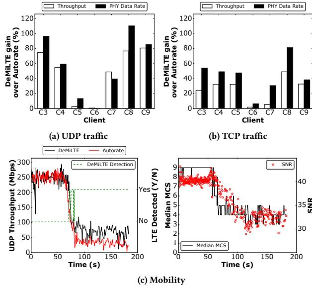
Figure 13: *DeMiLTE* with LTE below ED (AP2), on primary channel and 50% duty cycle.
