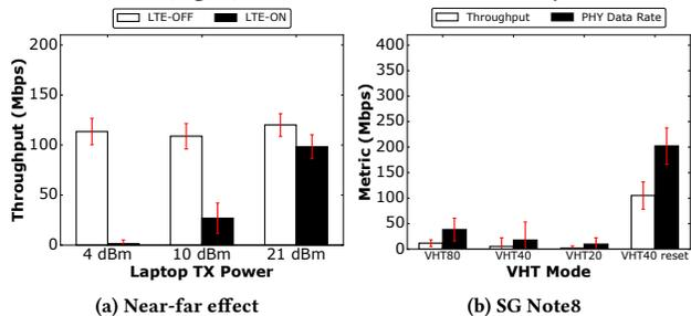
Figure 5: LTE-U on secondary channel, duty cycle 75%: Tests with different clients and VHT modes at location C7.
