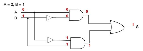
We can check all four possibilities this way. This circuit exactly and correctly duplicates the logic table created from our binary additions.
