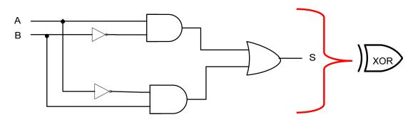
Notice that an xOR gate does correct binary addition for exactly one bit. BUT, we also know that the carry out information is ignored. Clearly, while this is a good first step it does not complete the job in creating a binary adder. More circuits are needed.
