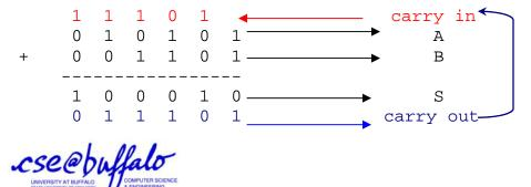
Notice, that while we think we are adding two numbers together, what we are really doing is adding 3-bits together (including our carry in) and getting an answer that is 2-bits (including our carry out). A complete or "full" adder performs operations on 3 bits,  $C_{in}$ , A, B. A full adder produces a Sum and a Carry Out.
