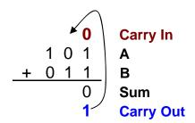
If you trace your values through the circuit above you can see how the circuit made up of a series of full adders solves the addition problem. Note the Sum which is the output of each column is what is written out to the computer output device (usually the monitor).
