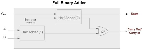
The full adder works is capable of adding any binary A with B and accurately keeping track of any Carry In and any Carry Out of that addition. When solving an addition problem, the initial Carry In is set to zero (0).
