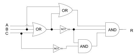
Now we can ask questions about the circuit. Let's let A = 1, B = 0 and C = 1. What is R? Just as before, write down the values on the circuit just before and just after each gate so we know exactly what the input and output from each gate becomes. In doing so we find that R = 0. Use the circuit below to test your work.
