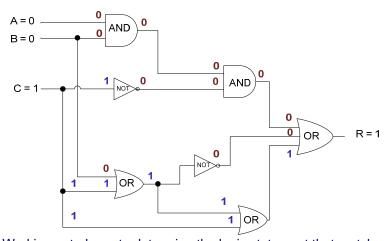
Working gate-by-gate determine the logic statement that matches this circuit.
