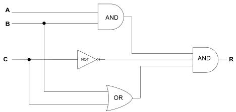
Examining the circuit above, we can ask a number of different types of questions. For example, we can be asked to determine the value of R, given information about A, B, and C. So, If A = 1, B = 0, and C = 0, what is R?
