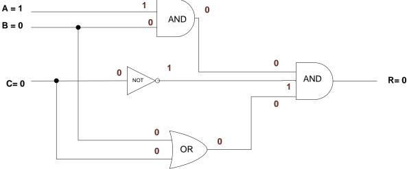
All circuits can also be evaluated using the appropriate logic statement or logic equation and a truth table to determine the various values of R. So, moving between circuits and logic statements is important.
