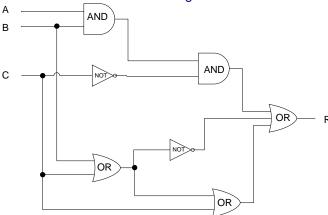
Trace the input and the output through each gate write down the values to determine R.
