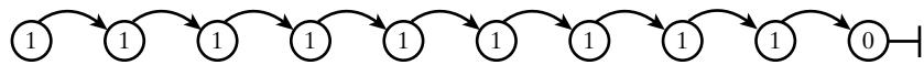
(a) Initial list with data values set to 1. Every processor knows the list element one place away.
