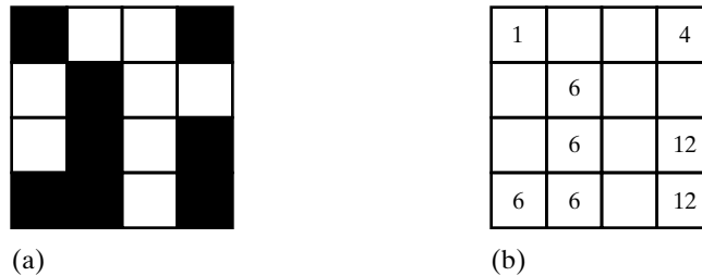
FIGURE 11-1 (a) A digitized 4 \times 4 picture. The interpretation is that the picture represents a black image on a white background. (b) The same 4 \times 4 picture with its maximally connected components labeled under 4-adjacency definition of connectedness. Every component is labeled with the minimum label of any pixel in its component. In this example, the pixel labels are given by their row-major indices, with values 1, \dots, 16 .
