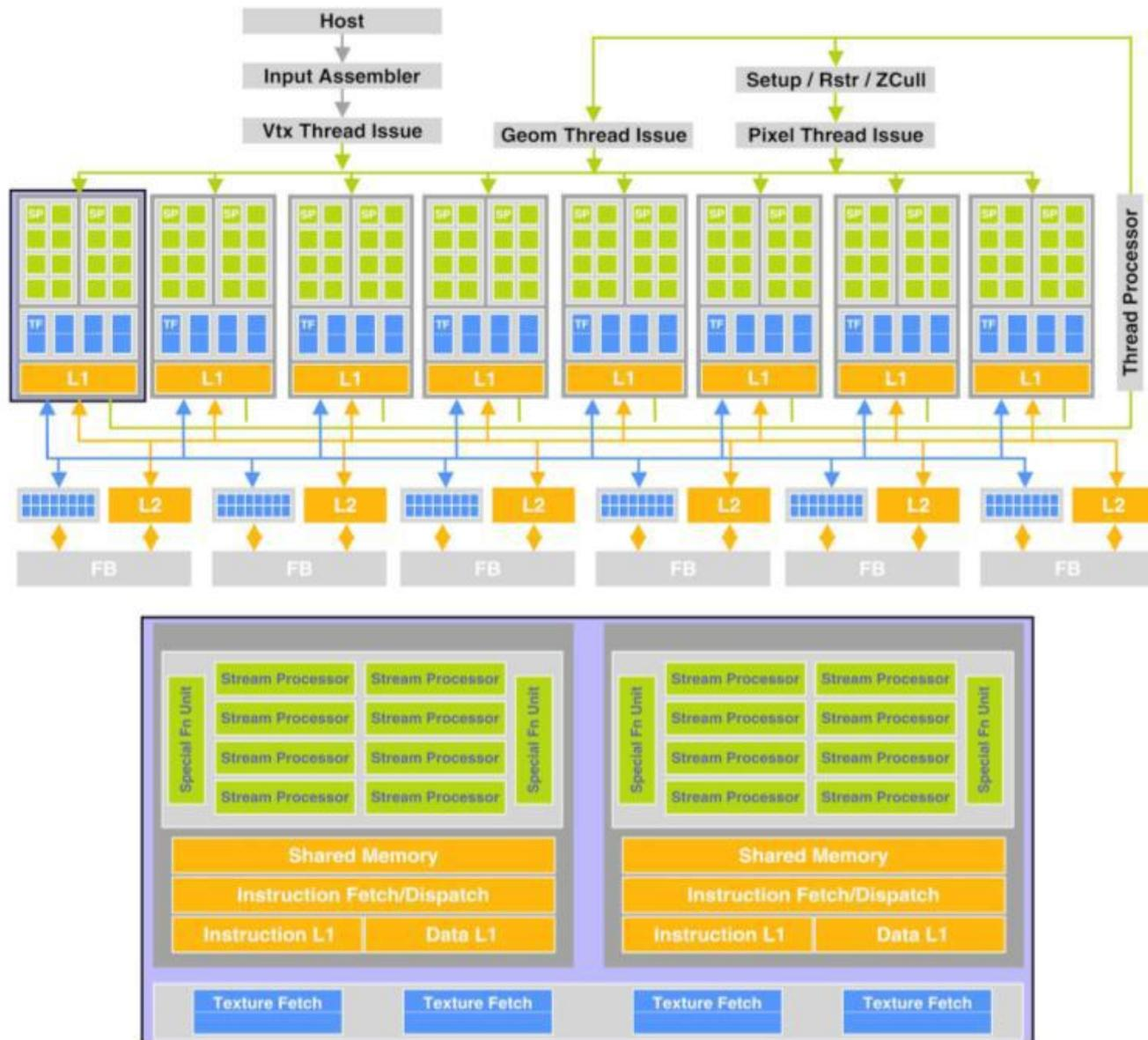
**Fig. 1.** Today, both AMD and NVIDIA build architectures with unified, massively parallel programmable units at their cores. (a) The NVIDIA GeForce 8800 GTX (top) features 16 streaming multiprocessors of 8 thread (stream) processors each. One pair of streaming multiprocessors is shown below; each contains shared instruction and data caches, control logic, a 16 kB shared memory, eight stream processors, and two special function units. (Diagram courtesy of NVIDIA.)
