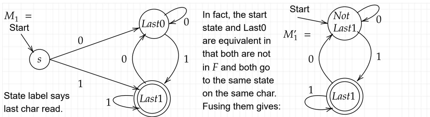
By popular demand, the table for  $M_1: M_1 = (Q, \Sigma, \delta, s, F)$  where  $Q = \{s, Last0, Last1\}$ ,  $\Sigma = \{0, 1\}$ , the start state is literally called  $s$ ,  $F = \{Last1\}$ , and  $\delta: Q \times \Sigma \rightarrow Q$  is defined by
