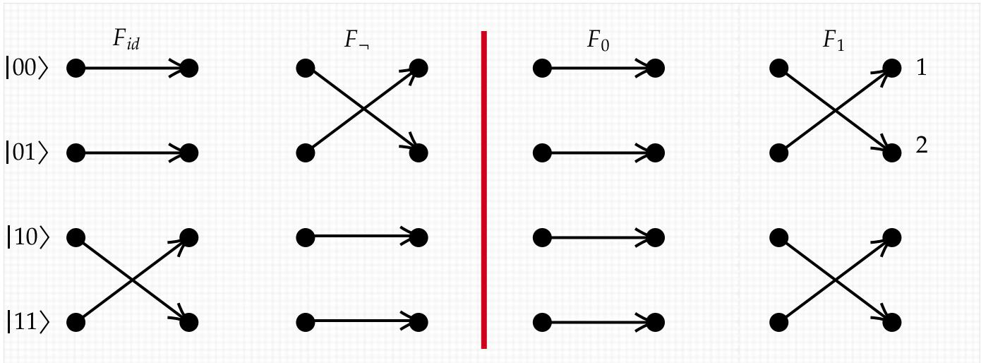
A quantum circuit, however, can make one query to an oracle gate for any of these four functions, and can distinguish a member of the first pair from a member of the second pair by the answer to one qubit after a measurement. The input is not  $|00\rangle$  but instead  $|01\rangle$ ; that is, the ancilla is initialized to **1**, not to **0**. Here is the wavefront ("maze") diagram of how it works:
