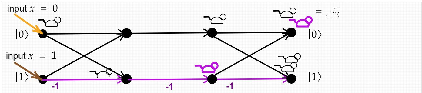
This time, when "Phil" starts running from  $|0\rangle$  at left, the "mice" cancel at  $z = |0\rangle$  and amplify at  $z = |1\rangle$ . And on input  $x = |1\rangle$  they output the basis state  $|0\rangle$ . The result is Boolean NOT, i.e.,  $\mathbf{X}$ .
