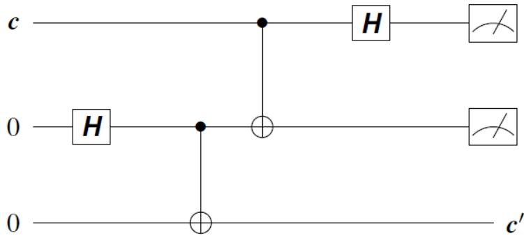
With this indexing, the start state is  $c \otimes e_{00}$ , which equals  $ae_{000} + be_{100}$ . After the first two gates, the state is
