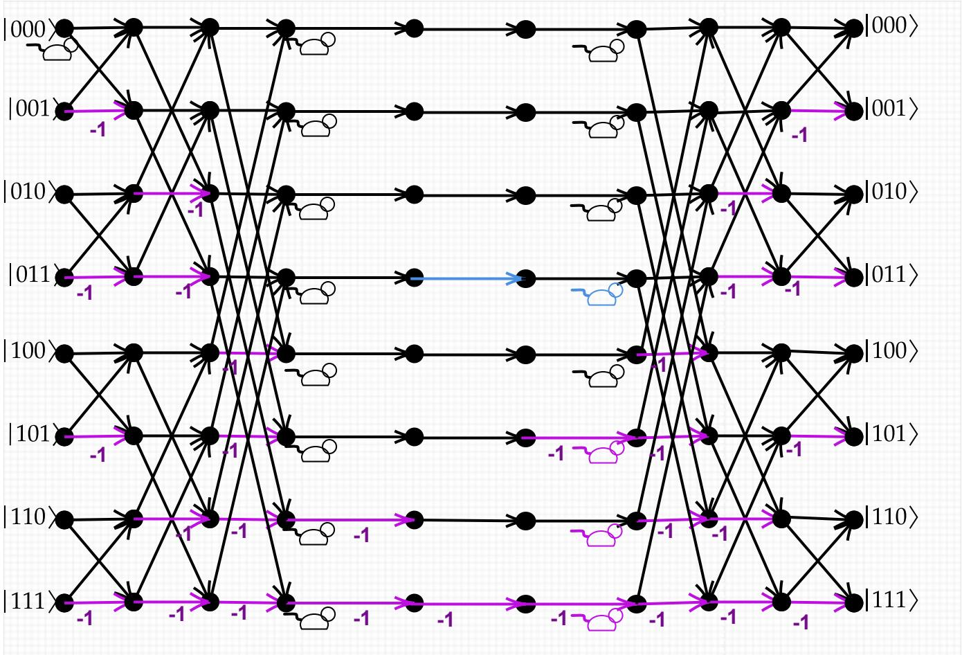
The only change was in the middle column, removing the  $-1$  from the row for  $|011\rangle$ . The middle column now "fires" only when all 3 bits are 1, i.e., for the component of  $|111\rangle$  in any state. This is the action of the double-controlled Z-gate, **CCZ** (which is really a triple control of a  $180^\circ$  phase shift). It is easy to diagram in a quantum circuit:
