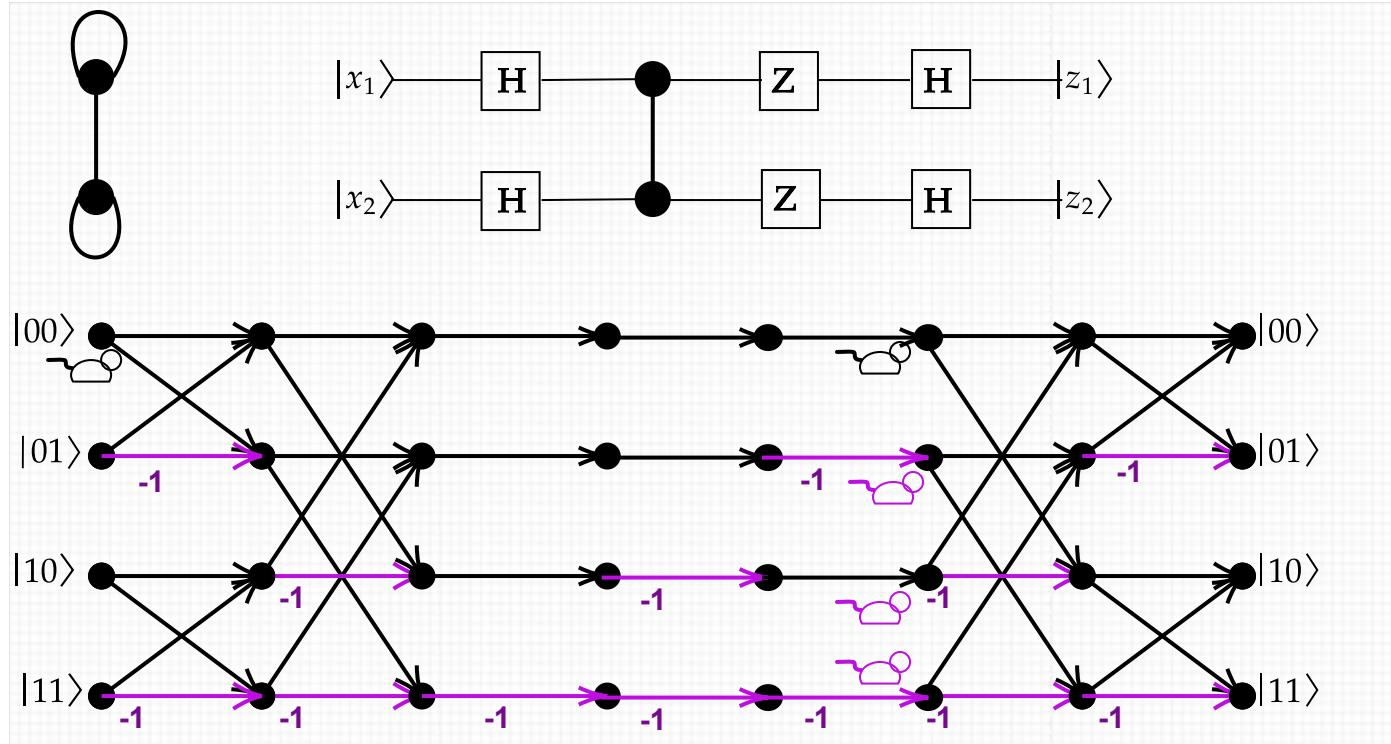
The  $-1$  phase shifts for the **Z** gates go on the basis states that have a 1 on line 1 or 2, respectively. Now the amplitude value  $\langle 00 | U_G | 00 \rangle$  is negative. Its sign does not affect the probability and the state still gives an equal superposition.
