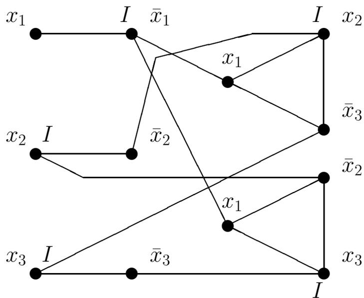
Figure 1: Construction in the proof of NP-completeness of INDEPENDENT SET for the formula  $(x_1 \vee x_2 \vee \bar{x}_3) \wedge (x_1 \vee \bar{x}_2 \vee x_3)$ . The independent set of size 5 corresponding to the satisfying assignment  $x_1 = \text{false}$ ,  $x_2 = \text{true}$ , and  $x_3 = \text{true}$  is shown by nodes marked  $I$ .
