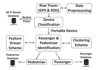
Figure 5: Trellis architecture. The raw GPS and RSSI is processed together to identify passenger and pedestrian. Passenger and pedestrian are sent to corresponding modules for further information extraction.
