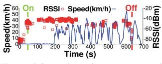
(a) An example data trace showing where a passenger gets on and off the bus.
