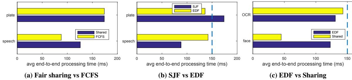
Figure 3: The impact of scheduling algorithms on the end-to-end processing time
