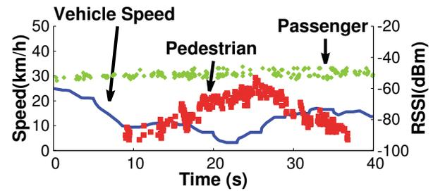
Figure 2: Different RSSI patterns between passenger and pedestrian.
