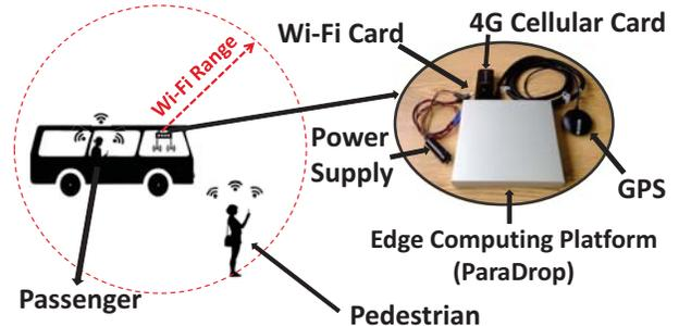
**Figure 1: The on-board edge computing platform.** The key challenge for Trellis is to determine whether an individual is located inside the vehicle (passenger) or outside of it (pedestrian). Based on the fact that pedestrians will eventually be out of monitoring range, Trellis solves this problem by observing device signal strength coupled with the vehicle’s speed of movement.
