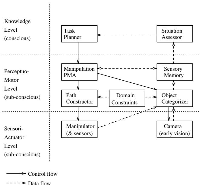
Figure 5: Schematic representation of the Robot Waiter GLAIR-agent.
