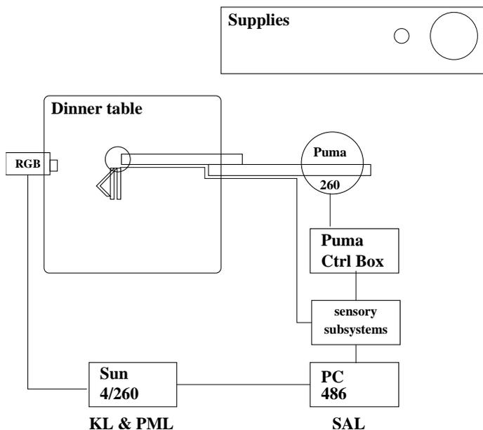
Figure 4: The Robot Waiter physical setup.
