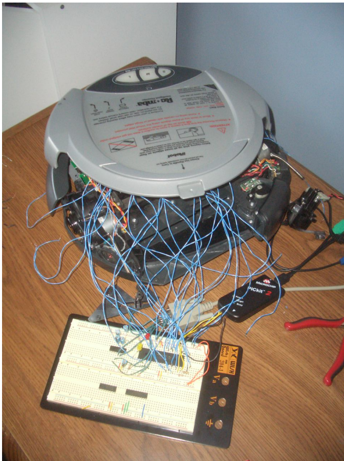
Fig. 2. The microcontroller wired to the robot.
