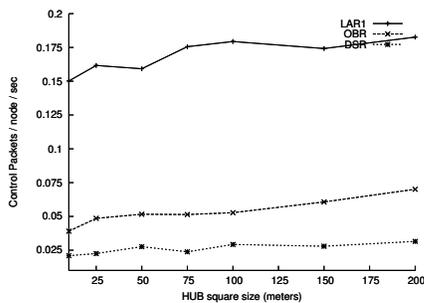
Fig. 16. Control Overhead vs. Hub Size
