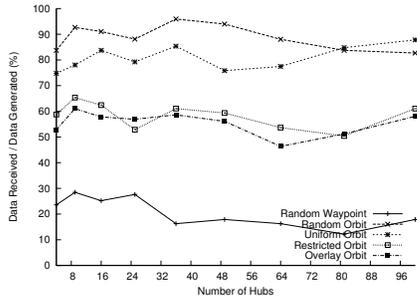
Fig. 12. OBR: Data Throughput vs. Number of Hubs
