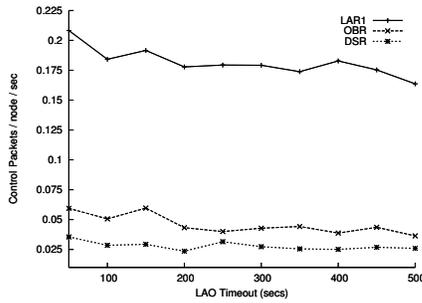
Fig. 19. Control Overhead vs. LAO Timeout
