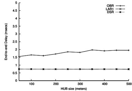
Fig. 17. End-to-End Delay vs. Hub Size
