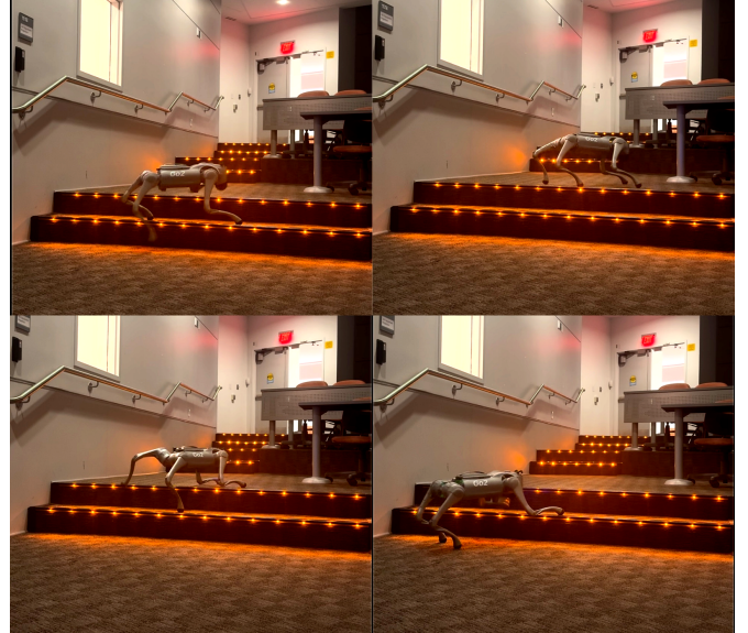
Fig. 1: Top: The Unitree GO2 robot begins ascending stairs approximately 16–17 cm in height. It first interacts with the steps to estimate their height, then adjusts its foot trajectory accordingly to initiate the climb. Bottom: The same robot performs a descent on the same staircase.
