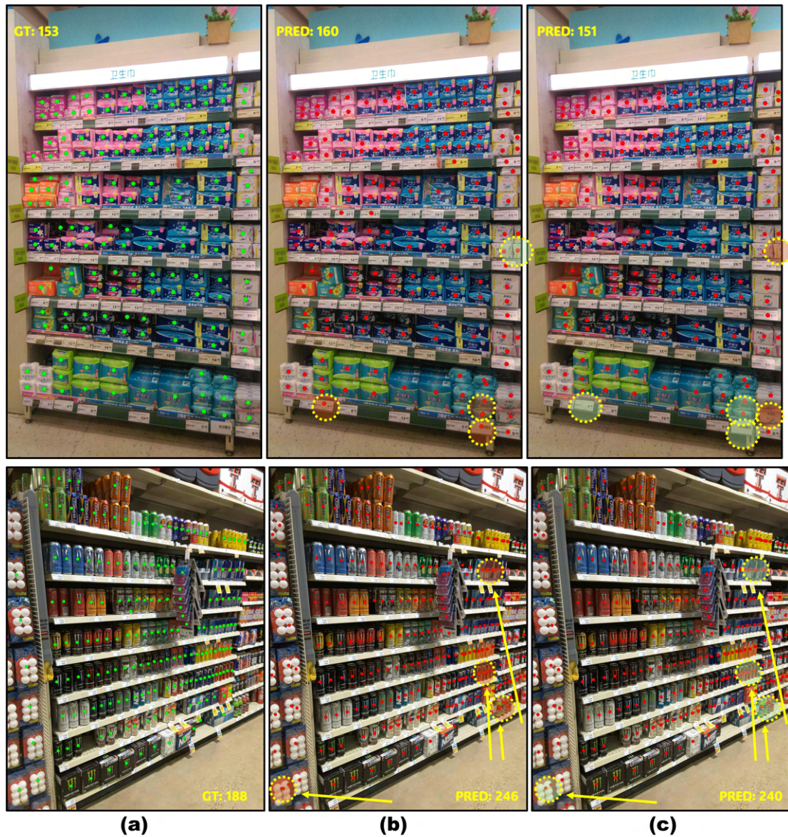
Figure 4.4: Qualitative comparison on SKU110K dataset. Each row displays the Ground Truth annotations (left), the Baseline predictions (middle), and our CoLC predictions (right). Regions where a model fails are highlighted with a red indicator (⊗) and corresponding successful with a green indicator (⊙).
