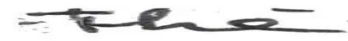
Fig. 3. The “Thee” bug. Before the context-mask fine-tune, “the” grows a fourth character because cross-attention is also attending to PAD. After a short fine-tune with the CANINE mask propagated through cross-attention, it attends only to real tokens and “the” is three characters again.
