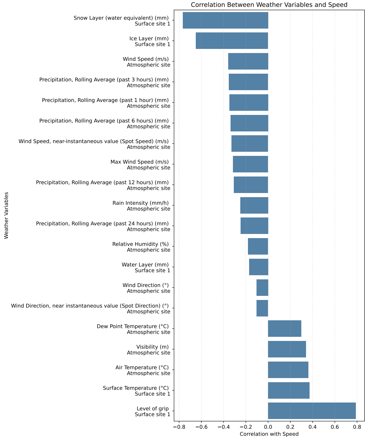
FIG. 4. Ground-truth Pearson correlation between observed speed and 20 road-weather features over the full study period. “Level of grip” (+0.78) and “Snow Layer” (−0.78) are the strongest signals. The 20 features visualized here define the feature subset used by the structural-consistency analysis (Fig. 7).
