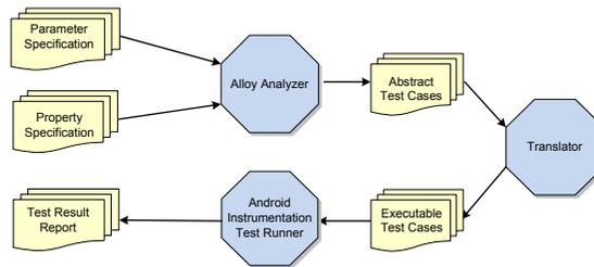
**Fig. 7.** A tool chain that supports MCTF
