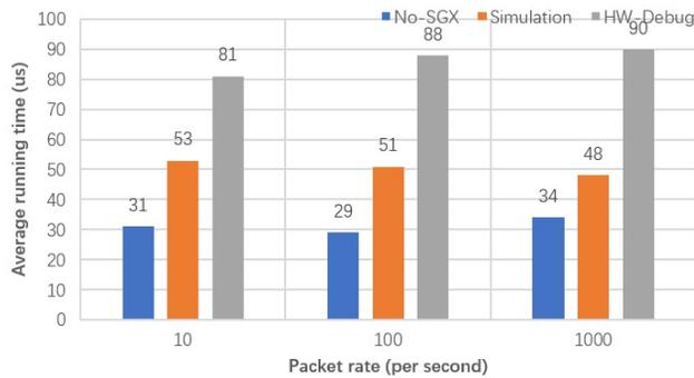
**Figure 3: Performance Overhead with SGX and without SGX**
