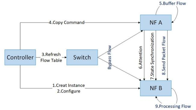
Figure 2: State Synchronization Process
