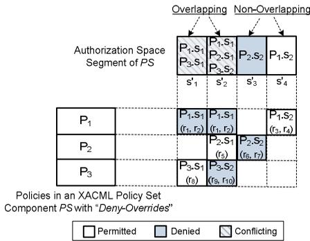
Fig. 10. Example of authorization space segmentation at policy set level for redundancy discovery and removal.
