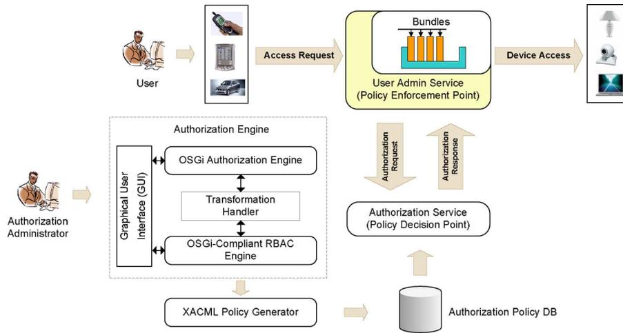
Fig. 8. Security-enhanced OSGi authorization architecture.
