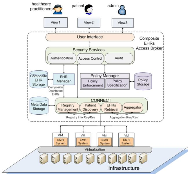
Fig. 5: System Architecture
