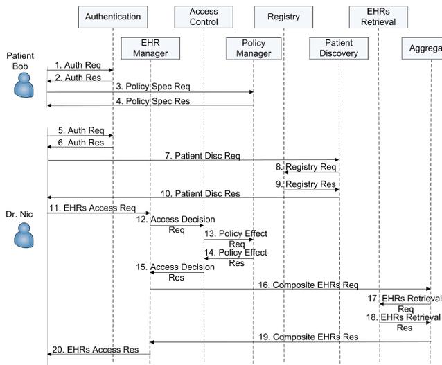
Fig. 6: System Workflow
