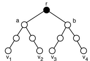
**Figure 3:** Solution returned by the algorithm for  $\text{RPP}/\infty/\text{req}$  problem for instance of graph  $G$ , where  $d = 3$ . There is no simple path between  $v_1$  and  $v_2$  in the solution
