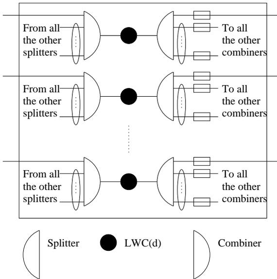
Fig. 3. A possible construction of the  $LWC(d)$  pool.
