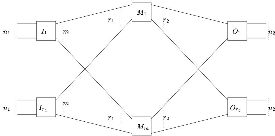
Figure 5.3: The 3-stage Clos network  $C(n_1, r_1, m, n_2, r_2)$
