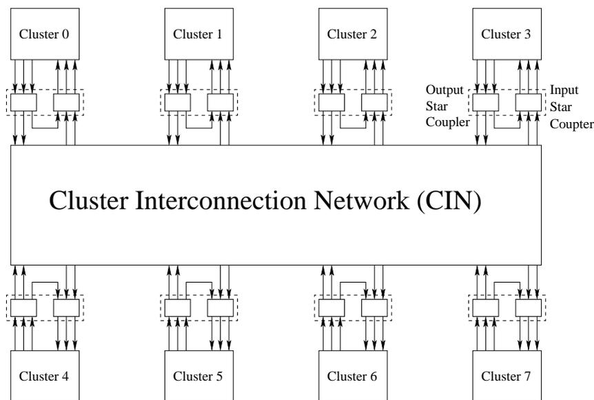
Figure 1.7: A clustered based optical interconnection network
