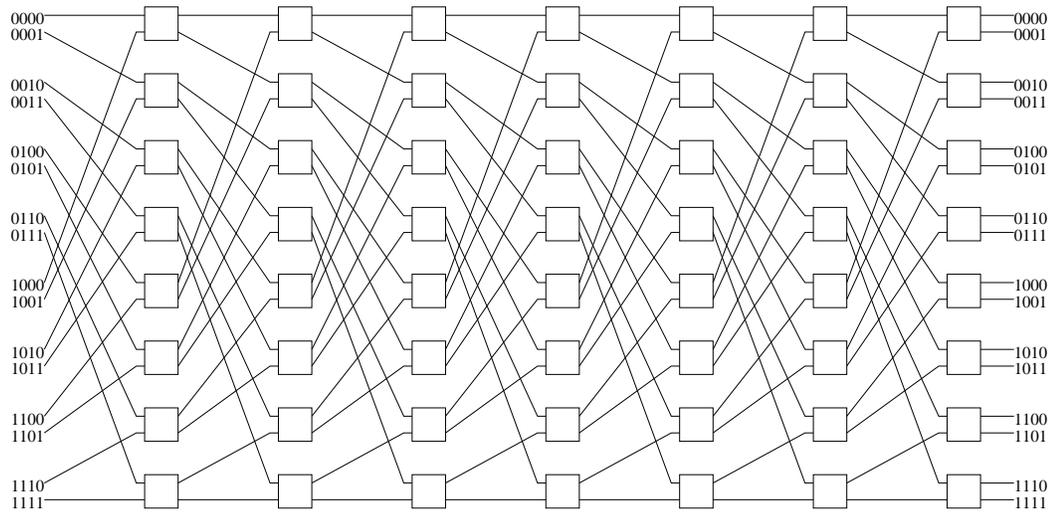
Figure 3.2: The 7-stage SE network for  $n = 4$ , i.e.  $(SE_4)^7$
