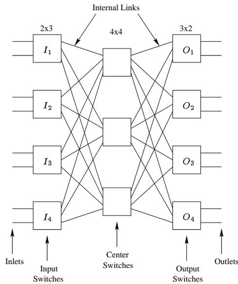
Figure 4.2: A 3-stage Clos network  $C(2, 3, 4)$
