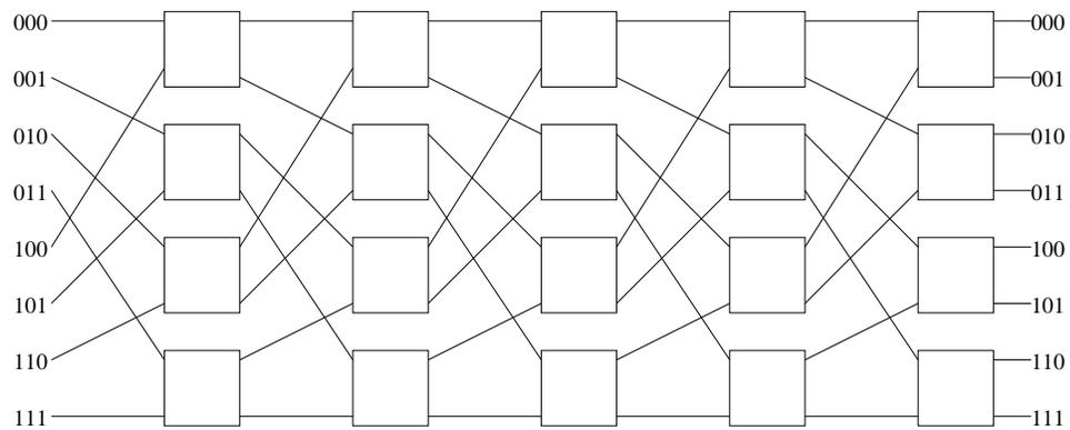
Figure 1.6: The 5-stage Shuffle-Exchange network  $(SE_3)^5$
