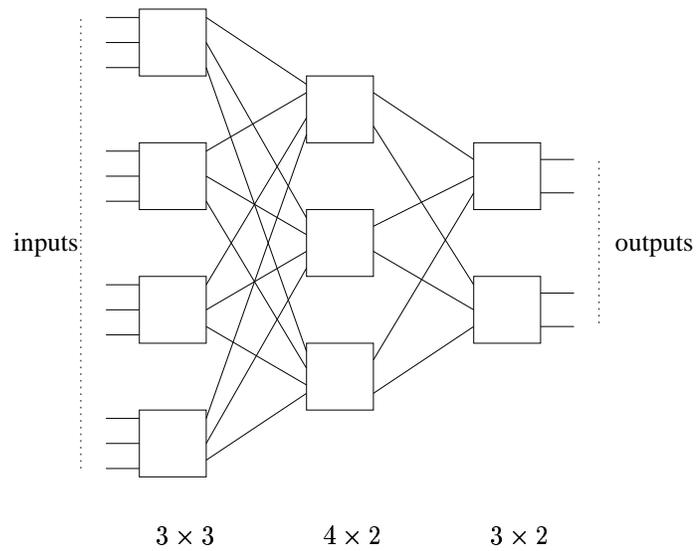
Figure 1.5: A 3-stage interconnection network
