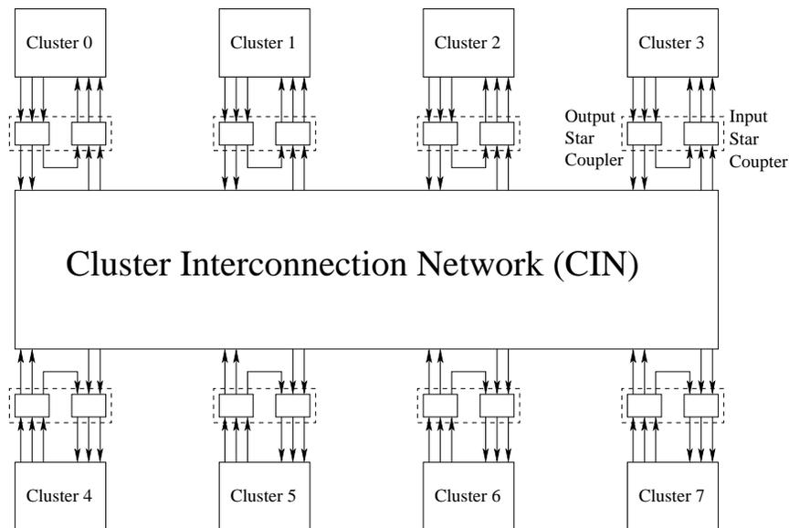
Figure 8.1: A Cluster-based Optical Network Topology
