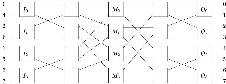
Figure 3.4: A redrawing of the  $(SE_3)^5$  network
