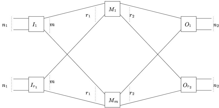
Figure 4.1: The 3-stage Clos network  $C(n_1, r_1, m, n_2, r_2)$
