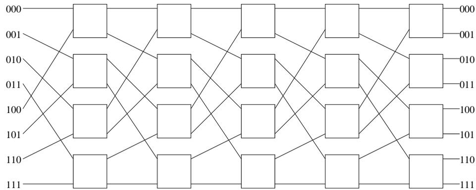
Figure 3.3: The 5-stage SE network for  $N = 8$ , i.e.  $(SE_3)^5$
