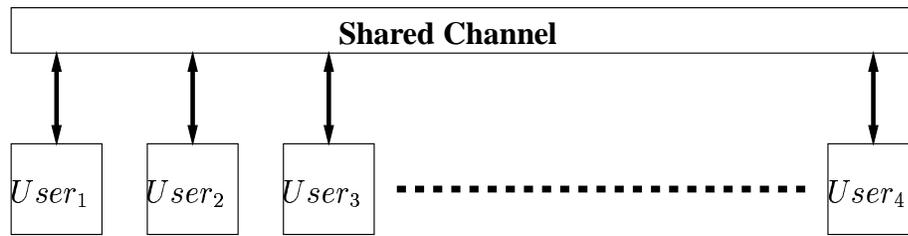
Figure 2.1: A generic model for multiaccess channels
