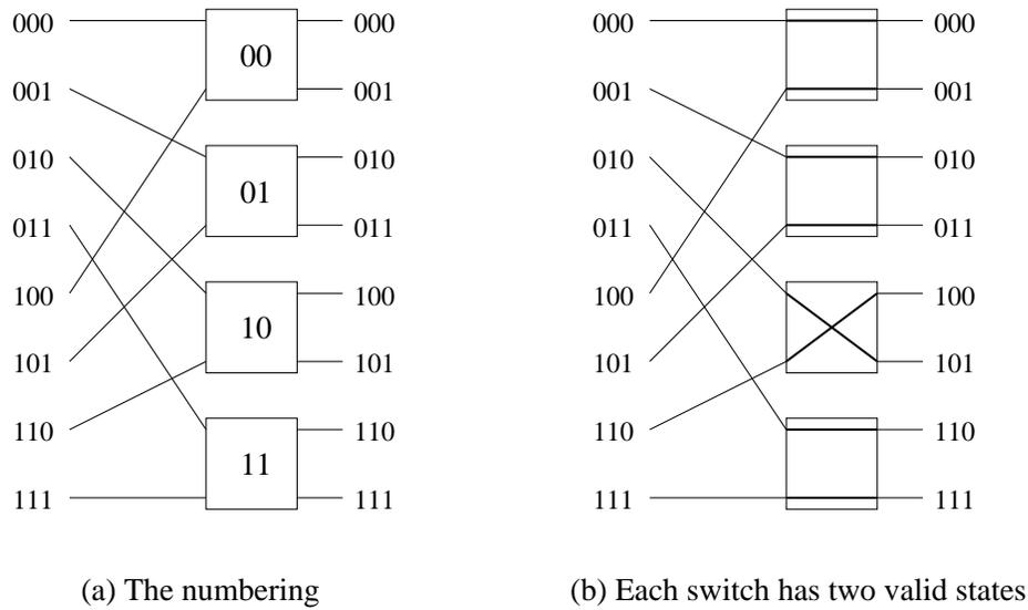
Figure 3.1: A Shuffle-Exchange stage with parameter 3:  $SE_3$
