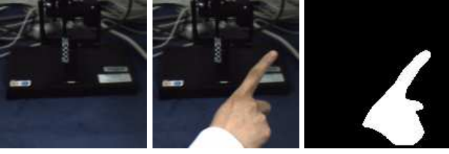
Figure 2: An example of background image (left), foreground image (middle) and segmentation result (right).
