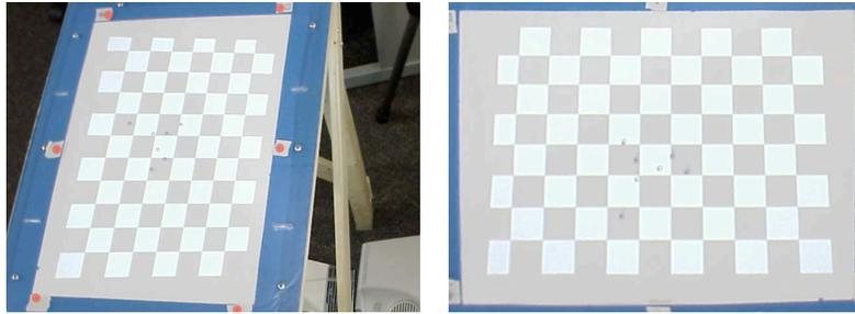
Figure 2.12: (left) The original image from one of the cameras. Calibration points are shown highlighted in red. (right) The same image after it has been rectified by  $H_i$ .
