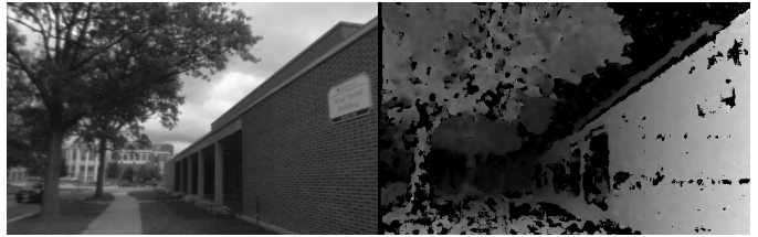
Fig. 1. A typical image with its disparity map. Invalid regions of the disparity map are in black.
