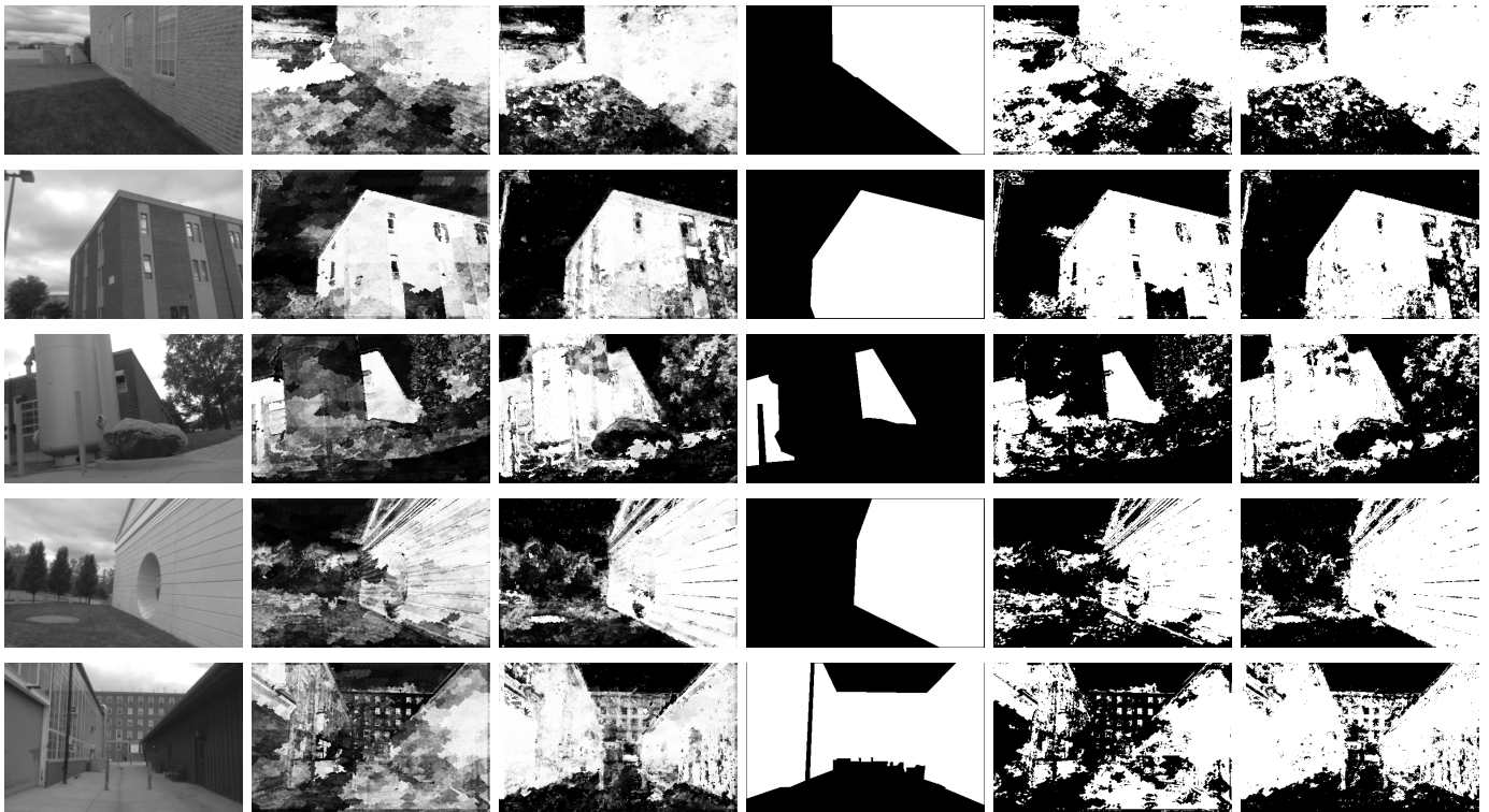
Fig. 4. Several examples of classification output. For each image set, the individual images are (L to R): Original Image, Standard BMA Probability, Image+Disparity BMA Probability, Ground Truth, Standard BMA Label, Image+Disparity BMA Label
