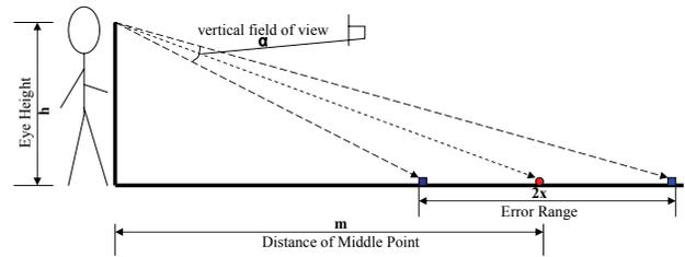
Figure 3: The size of one pixel on the ground plane. For an eye-height of 1.75m, a vertical FOV of  $38^\circ$  (matching our HMD), and vertical resolution of 480 pixels, the ground plane image of one pixel ( $2x$  in the figure) is 2.0cm at 7.5m and 4.7cm at 15m.
