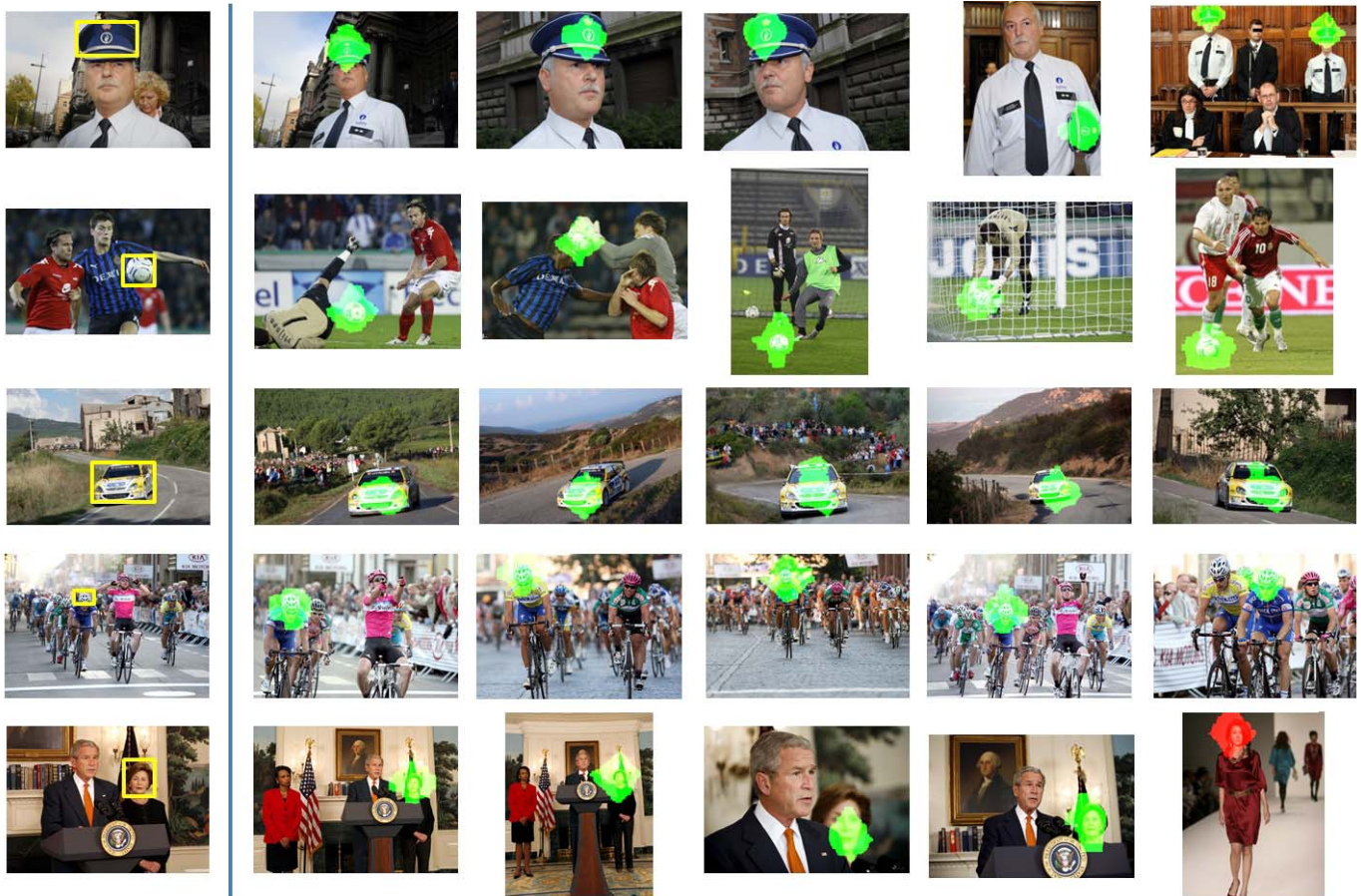
Fig. 15. Besides the logo queries, more general objects are tested by our search system. Here we give several examples for 5 general query objects: service cap, football, car, helmet and woman face. Similarly to Fig. 14, the queries are denoted in the yellow bounding boxes shown in the left column, and the selected results are shown in the right.
