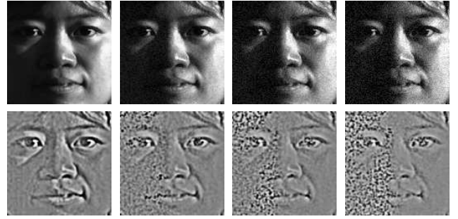
Fig. 2. The first row shows the sample images of CMU-PIE with additive uniform noise p = 0, 0.1, 0.15, 0.2 . The second row shows the photometrically normalized images.
