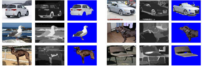
Fig. 5. Some sample results of our quick co-segmentation method. In spite of object not being so salient in the saliency map [20], the proposed approach is able to extract it.
