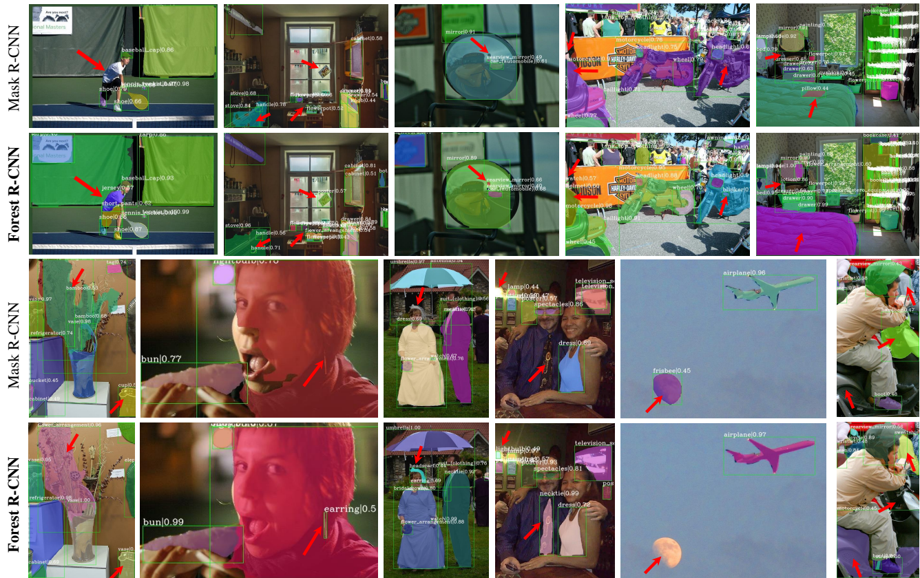
Figure 8: Mask R-CNN [16] vs. Forest R-CNN. Mask R-CNN exhibits more wrong classification and miss recognition. For neat visualization, we apply the NMS with threshold of 0.7 and filter out the predictions with scores lower than 0.4.
