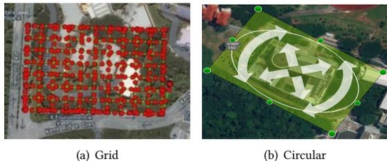
Figure 2: Camera positions for grid and circular flight.
