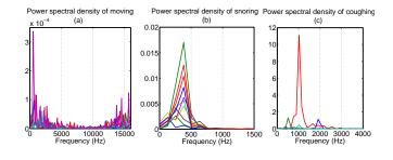
Figure 2: (a), (b) and (c) show the power spectral density of typical moving, snoring and coughing events, respectively.
