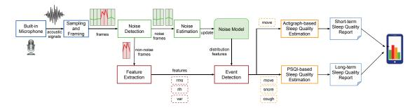
Figure 1: The architecture of iSleep system.
