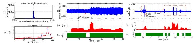
Figure 8: (a) The histogram of sound intensity of a 4-second body recording containing standard deviation of each frame. The acoustic data is collected by iPhone 4s for a duration of 4 seconds.
