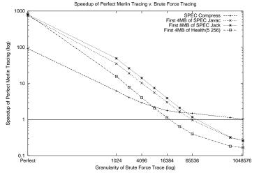
Figure 7: The speedup of Merlin versus Brute Force trace generation. Note the log-log scale.
