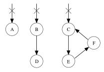
Figure 2: Objects A and B are reachable until their last incoming reference is removed. Object C is last reachable when an incoming reference is removed, even though it has others. Objects D, E, and F are reachable until an action that does not affect their incoming references.
