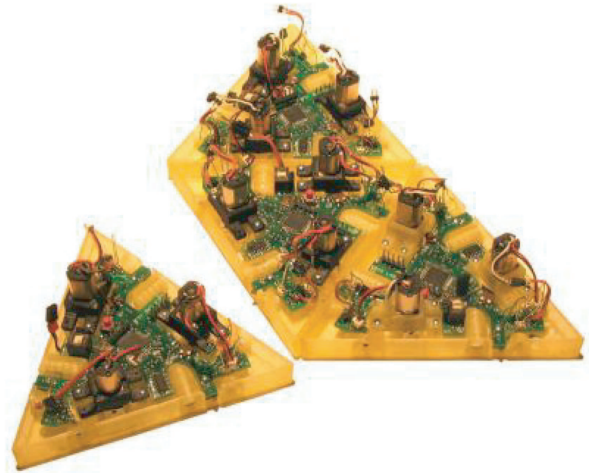
Fig. 1. Four programmable parts partially assembled into a triangle. The parts bind upon random collisions and communicate via IR, deciding whether to remain bound or to detach. A graph grammar stored on the microcontroller of each part determines the ultimate global structure that will emerge. The parts are not self-motive but instead are “mixed” on an air table by overhead oscillating fans.
