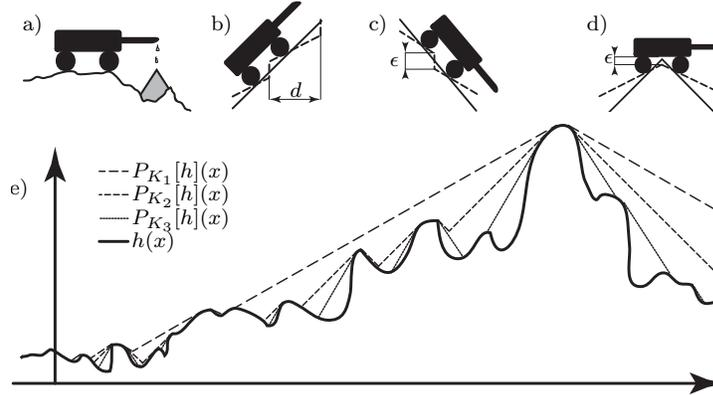
**Fig. 2** Parameter Geometry. (a) Robot making an amorphous deposition. (b,c) Relation of  $K$  to the maximal steepness a robot can climb and descend, (solid) without discontinuity (dashed) with discontinuity. (d) Relation of steepness  $K$  to the required ground clearance to drive over the apex of a cone. (e) A height function on  $h \in \mathcal{Q}^+$  and its projections onto Lipschitz functions with different parameters  $K_3 > K_2 > K_1$ .
