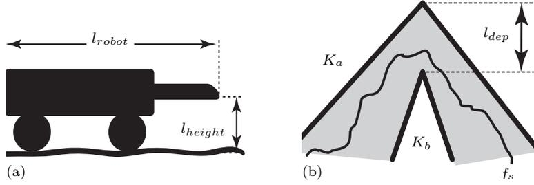
**Fig. 4** Physical parameters. (a) Relevant robot dimension based on the prototype shown in Fig. 1(b). (b) Parameters for bounds of an arbitrary deposition shape function.
