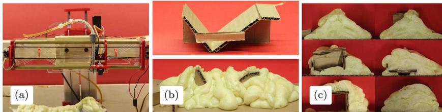
**Fig. 6** Scanning foam deposition mechanism. (a) A scanning carriage holds a downward facing IR-distance sensor and mixing nozzle. Pressurized foam precursors are delivered to the nozzle by flexible tubing. (b) Top, Initial obstacle before leveling deposition. Bottom, final structure after deposition episode. (c) Cross sections of final structure. Each leveling deposition episode represents one cone-like deposition in Alg. 2.
