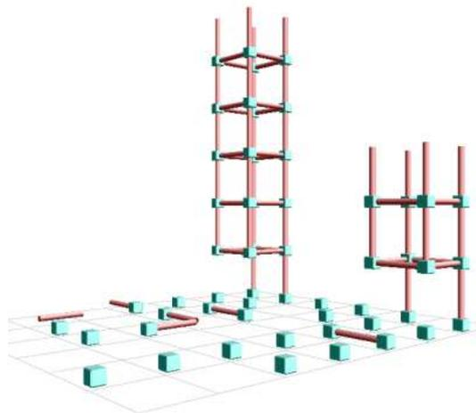
Fig. 1. Simulation of a decentralized multi-robot system, building two towers. Each square on the bottom layer represents a robotic module that can manipulate the two types of building materials trusses (red) and nodes (blue). Here, the construction area in the back receives building materials at twice the rate as the one in front. As a result the back tower is higher.
