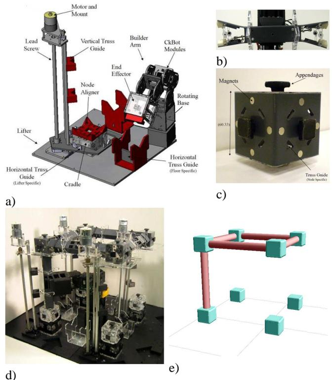
Fig. 2. The Factory Floor testbed. a) Schematic representation of a Factory Floor module. b) Picture of truss type raw material. c) Picture of node type raw material. d) Picture of four modules assembling a two layer structure. e) Picture of same structure in simulator. Module components are omitted for clarity.
