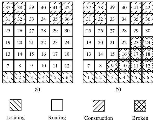
Fig. 3. Layout of construction program. The modules that run the loading program also run the routing program. Construction area 1 consists of modules 31, 32, 37, and 38, while construction area 2 consists of modules 35, 36, 41, and 42. The routing program is the same as for all modules except for the border modules of the two construction areas as shown in Fig. 5. a) Programs during normal operations. b) Failure scenario. Broken modules do not pass any raw materials.
