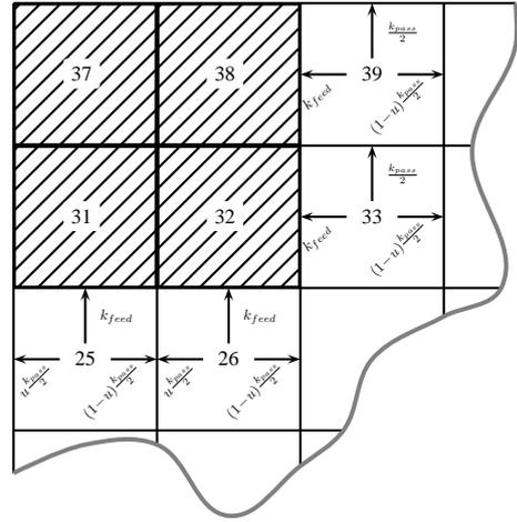
Fig. 5. Border modules of construction area 1. The expected value of the feed rate into the target area is a linear function of the expected occupancy time for the border modules. The modules 25,26,33, and 39 pass a raw material (node or truss) into the target area at rate  $k_{feed}$ . If  $\mathbb{E}s_i$  denotes expected value of module  $i$  possessing a raw material, then the expected feed rate is  $k_{feed} \mathbb{E}s_i$ .
