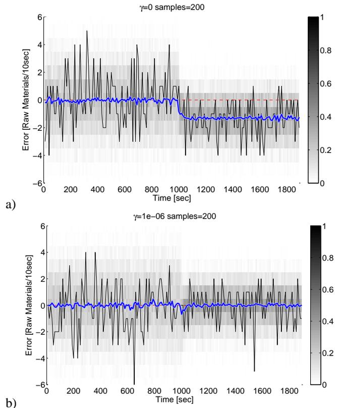
Fig. 6. Routing raw materials with the failure shown in Fig.3b at  $1000sec$ . a) Difference in routing rates in open-loop. The fraction of trajectories at a particular value and time is indicated by the grey shading, showing the noise in the system. A sample trajectory highlighted in black and the thick blue line is the empirical ensemble mean. b) Difference in routing rates for the closed-loop controller with  $\gamma = 1e - 6$ .
